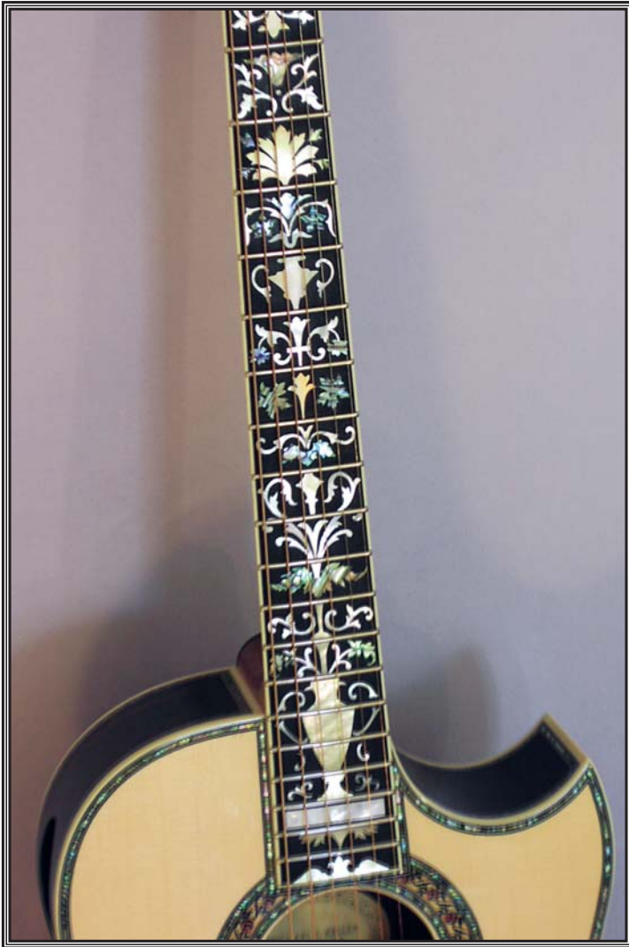
Classic Harwood design from Andy DePaule's Luthier Supply, cut in Vietnam out of top quality paua abalone, and modified and inlaid into the Nigerian Ebony fingerboard by Michael Keller. Has a custom compound radius fingerboard, nickel frets, and a 24-inch custom scale.
