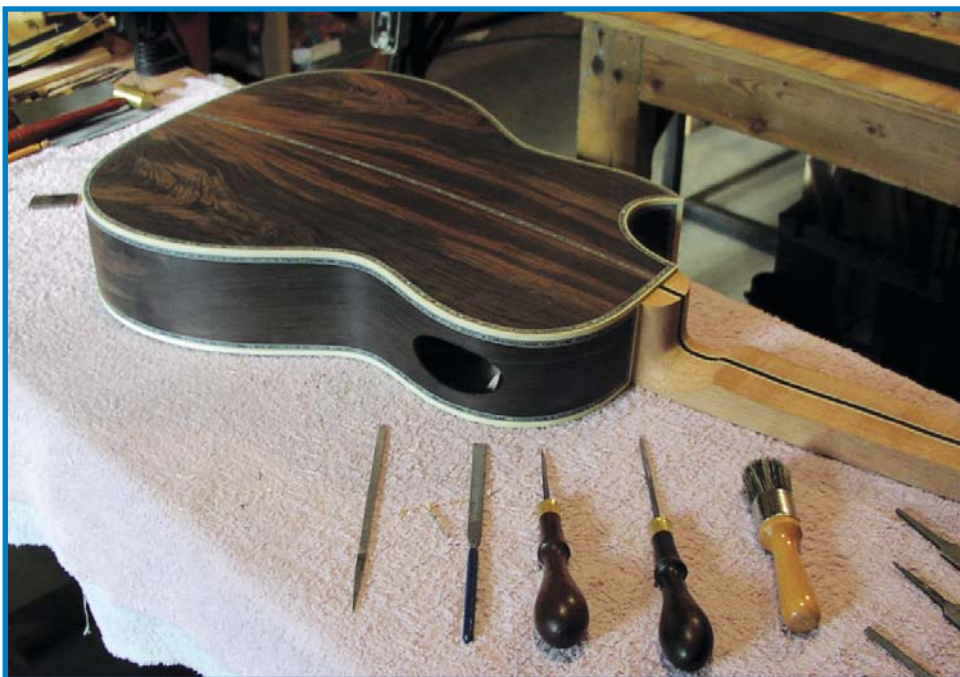
A masterpiece in the making. Note the attached neck is still square, and awaits the final shaping to the designated radius dimensions – very critical to the instrument's playability. The size and location of this sound port make a huge difference in the volume and how this instrument sounds to the player.
